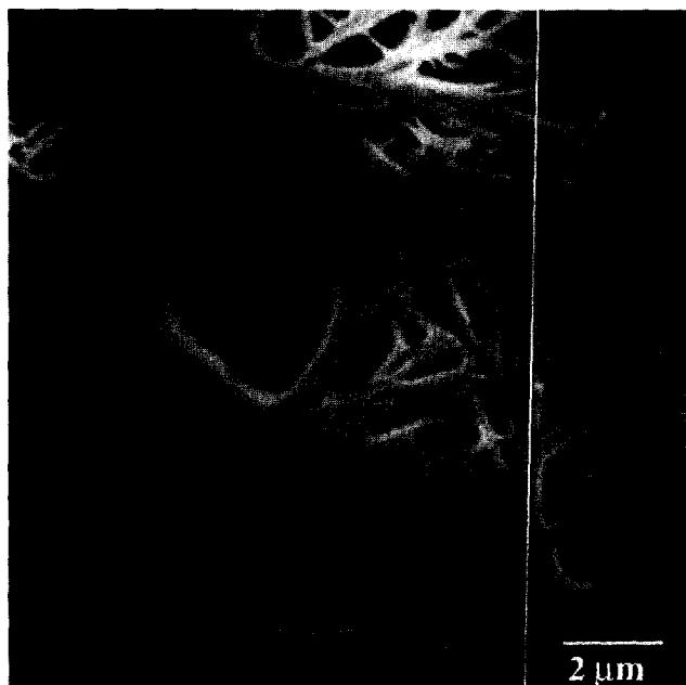
Figure 6 Bundles of s-PS in a-PS/s-PS blend. SEM image, amyl acetate etched sample
